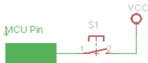
So, if the button is pressed, the 3.3V Vcc will be directly connected to the MCU Pin making it sense 3.3V and reads logic 1. Good? No! What happens when the button is not pressed? Is the MCU Pin going to read 1 or 0? Nobody knows. It is called a *Floating Pin*.
